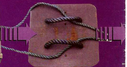
Simultaneously pass the tie ends under the board loops from the outside
