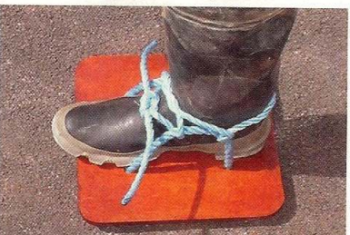
7. Pass the rope ends under the loops and tie off over the instep with a reef knot
